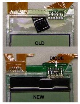
The diode, if present, is soldered across the LCD Connection pins.
